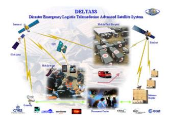
Mobile Teams, Permanent Center (PC), Mobile Field Hospital(MFH) and Reference Hospital (RH) are interconnected via several satellite systems with different bandwidths. Additionally terrestrial communication channels support the data exchange between PC and the RH <sup>14</sup>
